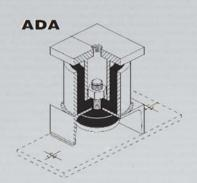
All-directional acoustical pipe anchors, consist of two sizes of steel tubing separated by a minimum 1/2" (12mm) thickness of 60 duro or softer neoprene. Vertical restraint shall be provided by similar material arranged to prevent up or down vertical travel.
